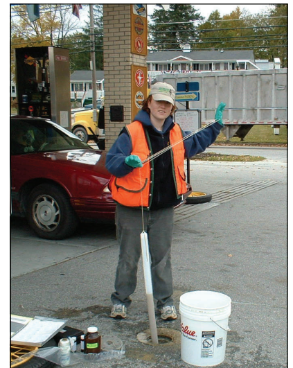
Monitoring well sampling.
