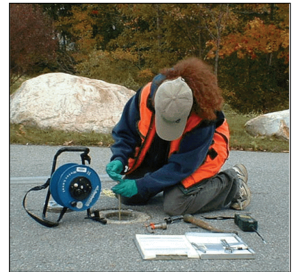
Groundwater level measurements.
